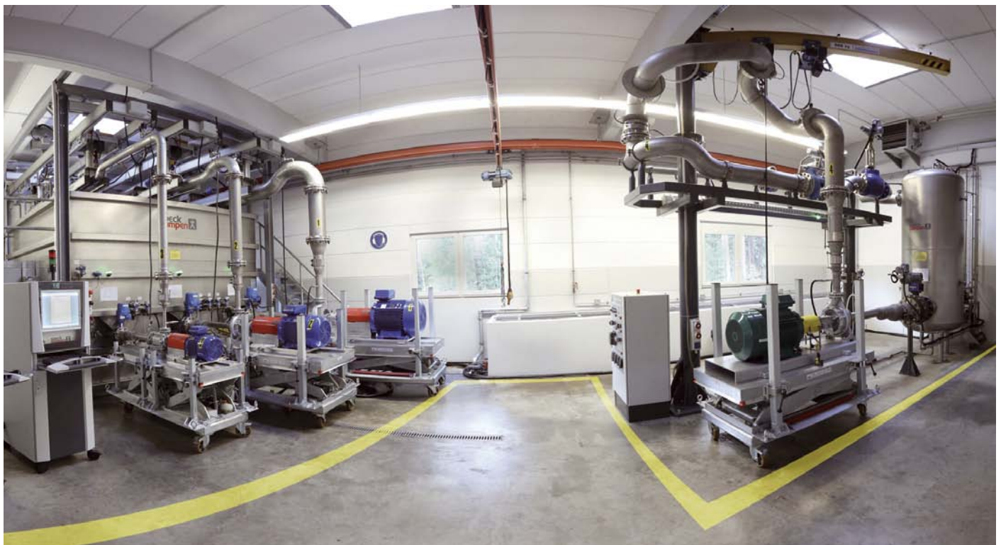
Computer-controlled and fully automated test stands on the premises of Speck in Roth.
