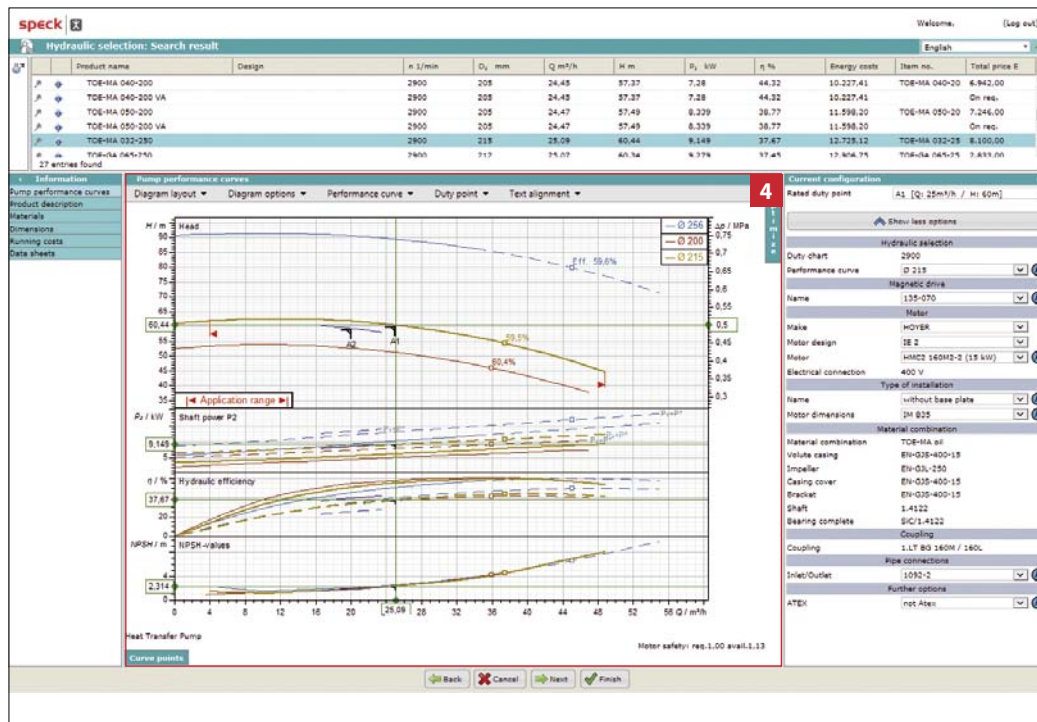
Characteristic curve depending on hydraulic selection
